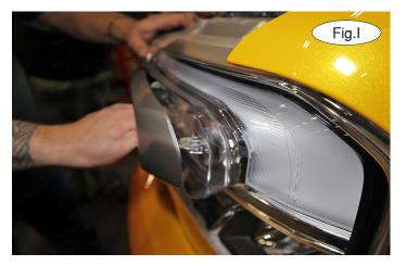
7. With the assistance of another person, use a flathead screwdriver to release the retaining clip on each side (Fig.H). Once it is loose, release three retaining clips on each headlight bezel (Fig.I) and then very carefully pull out to remove the fascia. Disconnect the passenger side wiring harness and set the fascia aside for now.
