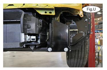
15. Then, using the drawing on page 1 as a reference, locate the driver's-side specific brace and place the upper mount with the welded spacer over the exposed mounts (Fig.T). Place Loctite on the factory nut and two factory 13mm bolts removed in the previous step and then replace them (Fig.U). Tighten the hardware to the factory specifications.
