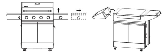
**3.** With two people, line up the Grill & Prep Cart on the side of the Anaheim 4-Burner Gas Grill, ensuring the doors are facing the same side, and press the cart onto the brackets attached to the brackets on the burner box of the grill.
