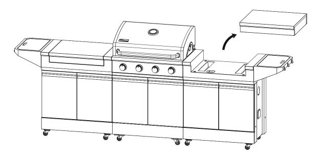
**6.** Place your portable unit on your Grill & Prep Cart, threading the gas hose through the center access hole.
