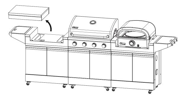
9. Place the portable grill into the chassis.
