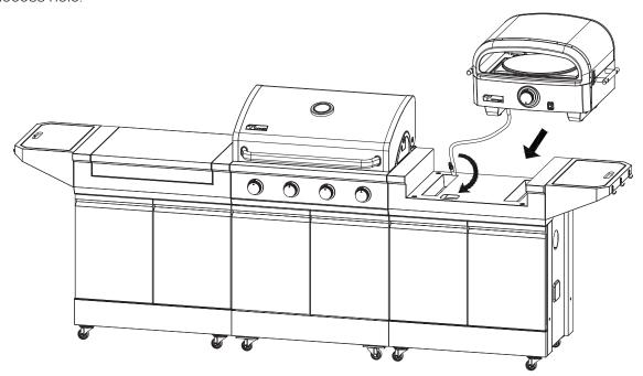
7. Thread the gas hose through the side panels and connect to the "T" gas hose assembly inside the main cart of the Anaheim 4-Burner Gas Grill.
