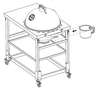
Place the collapsible trash bin onto the bolts on the right side of the charcoal kettle cart.
