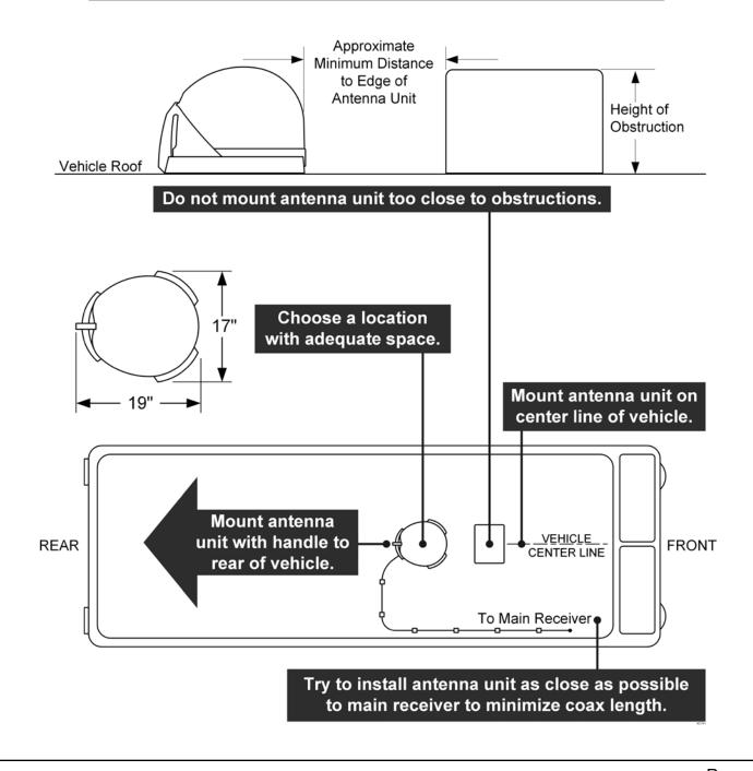
The installer is responsible for determining the most appropriate fasteners to secure the antenna unit to the roof. Depending on the roof material, fasteners such as lag screws, well nuts, sheet metal screws, toggle bolts and T anchors may be used, and should always be used in combination with a **roof-compatible sealant**.
