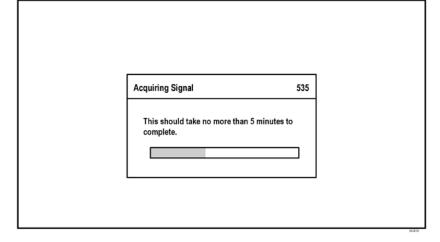
After your receiver has acquired the signal, the program guide will download. This may take up to 10 minutes to complete (potentially longer if an external hard drive is connected).
