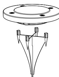
3. Align the 2 pins on the longer ground stake with the 2 remaining holes on the light. Push the longer ground stake through the slot of the shorter ground stake and insert into the light.
