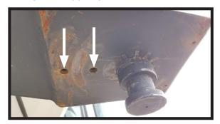
2. Using those bolts. Install the Demco Locking Plate into the two threaded holes that are directly behind the Turning Point king pin.
