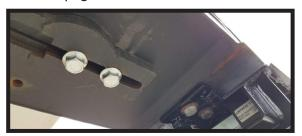
7. The two 5/8" serr. head Grade 5 bolts that come in the kit may be used to fasten Lipperts wedge back to the storage location on the pin box. The two serr. nuts that come in the kit will not be used.
