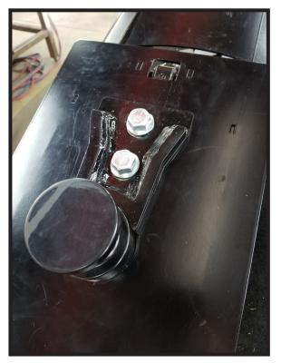
4. Place the 5/8" Grade 5 bolts and 5/8" nuts onto the locking plate as shown. Torque the bolts per the **BOLT TORQUE SPECIFICATION CHARTS** located on page 2.
