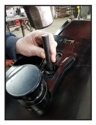
Make sure the locking plate does not move. Mark the holes that need to be drilled with a center punch.
