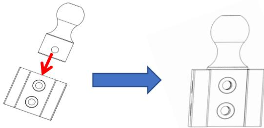
a. Align the hitch ball hole with the center of the bracket hole
