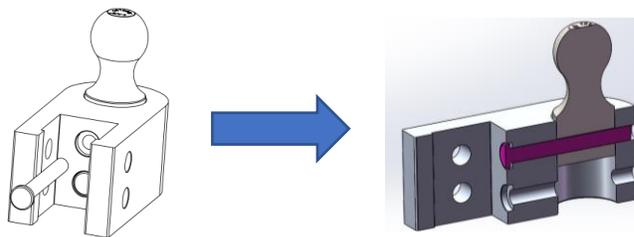
**Step 3: After installing hitch balls to adjustable section. Slide the adjustable section onto the aluminum drop at desired height and secure with the locking hitch pin and standard hitch pin. ALWAYS use both pins to secure adjustable section to the drop.**
