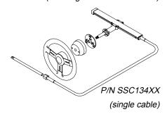
Traditional SeaStar Solutions mechanical steering is still the choice for sterndrives, inboards and other power assisted applications. It's just right for power steered boats in which No FeedBack™ systems are not required. Our new Rack features the precision and comfort of four turns lock-to-lock with a cable and helm that install easily from behind the dash. In single cable configurations, this is the best 4-turn choice for power-steered boats.
